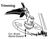
SCALPING - The scalping technique removes unwanted vegetation down to the ground. Hold the bottom of the trimmer head about 3 in. (8 cm) above the ground and at an angle. Allow the tip of the line to strike the ground around trees, posts, monuments, etc. This technique increases line wear.
